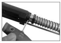
11) Remove the barrel nut locking screw. Note: There are two threaded holes on the barrel nut but only one set screw is used for purposes of locking the nut in the clocked position.
