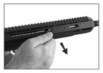
**4)** Pull out the charging handle by firmly holding on to it.
