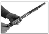
**15)** Slide off barrel nut, escutcheon and recoil spring.
