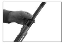
**9)** Remove the gas system locking nut in the clockwise direction.
