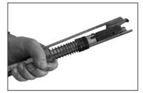
**14)** Push bolt carrier toward the barrel hood compressing the recoil spring. Swing the bolt carrier away from the barrel hood and remove the bolt. Everything will be free at this point.
