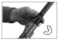
**10)** Twist off the gas piston cup and the rest of the piston system can be removed
