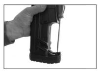
**6)** Remove the Philips screw that holds the back stock pad in place.
