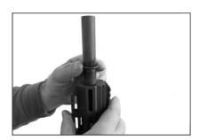
**3)** Remove the O ring if it does not remain in the groove of the handquard nut.
