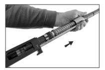
13) Remove the barrel from the receiver
