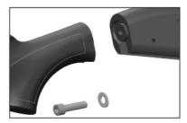
11) The stock can be pulled back away from the receiver. Note: there is not need to remove the stock for maintenance or cleaning, only if you wish to replace it with a different model.
