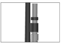
**3)** Remove the barrel nut by rotating it in the counter clockwise direction
