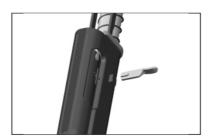
**5)** Remove the charging handle by aligning the key slot on the bolt with the key on the charging handle.
